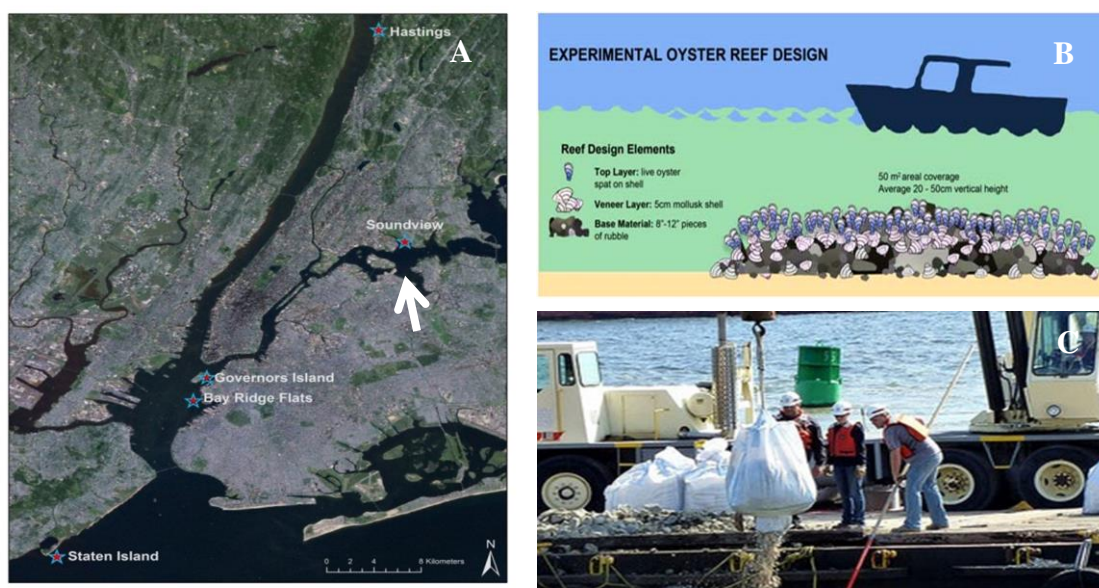
Figure 1. A., Location of present project at Soundview Park (white arrow) and four other experimental ORRP oyster reefs constructed in 2010; B, schematic of individual reef design (upper right); and C., photo of clam shell foundation being deployed at the Governors Island site.
