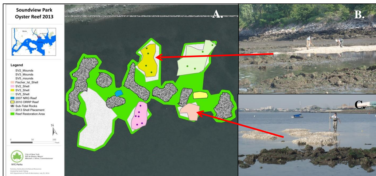
Figure 9. A: As-built reef base configuration and spat-on-shell deployments showing major components and spatial relationship to previously constructed Park reef (small blue polygon “2007 NRG Reef”), ORRP reef (small light yellow polygon “2010 ORRP Reef”), and rock bottom areas present before reef base construction (gray mottled polygons “Subtidal Rocks”). The overall approximately 1 acre restoration area is depicted by the green polygon. Photos B and C (June 2013) are of two shell mounds the day after construction. Manual spreading of shell in B. was used in order to get more even distribution of shell (see text for details). Red arrows denote the locations of photos on the polygon map.
