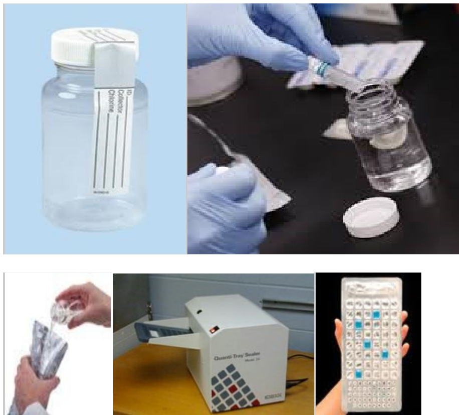
Figure 1. 120 ML sample bottle and major components to prepare Quanti-Tray 2000
