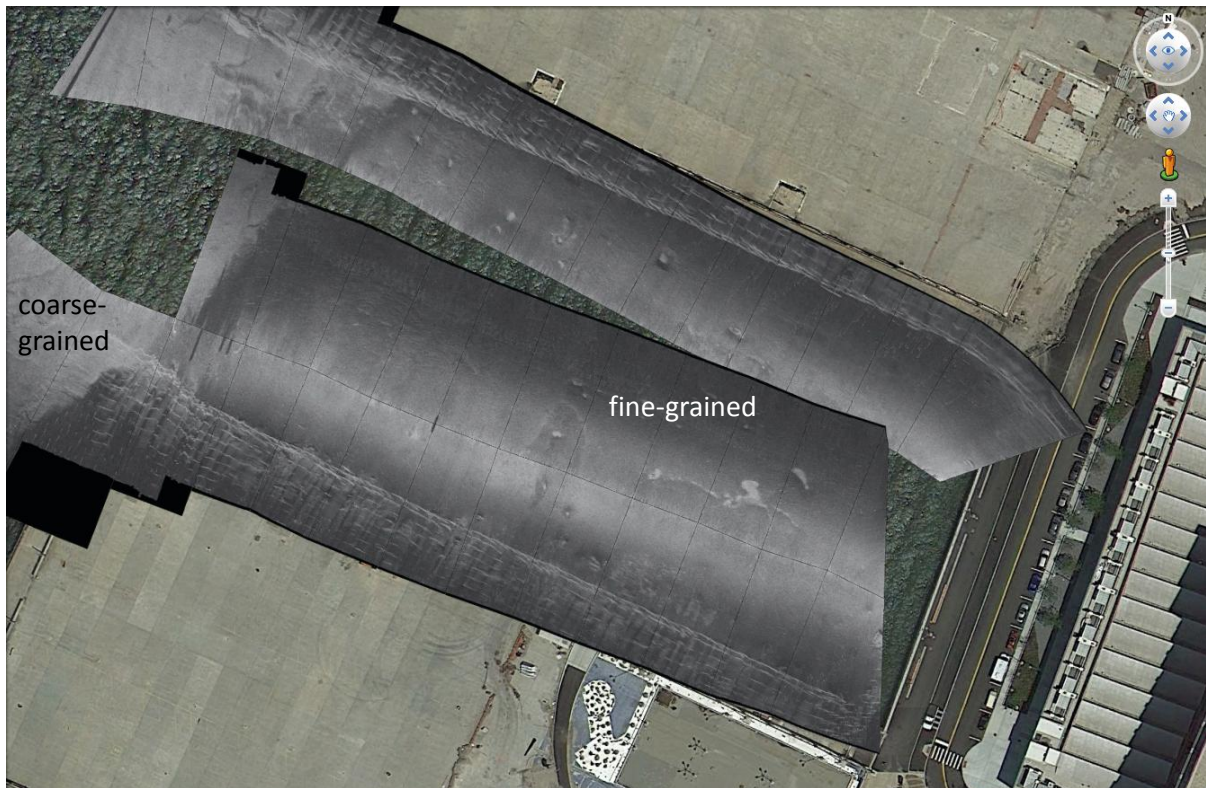
Figure 3.7. Sidescan sonar image of the slip at Brooklyn Bridge Park on July 29, 2013. Fine-grained sediment appears dark, and coarse-grained sediment and other bottom features appear lighter. Grazing angle with distance from the survey vessel also matters, with brighter return along the centerline of the vessel track.
