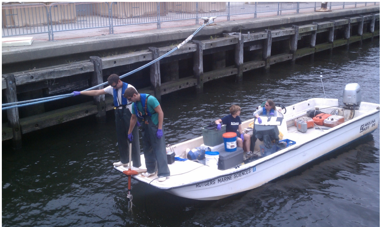
Figure 4. Sampling with DIDSON on a pole mount at Pier 6 with the barge absent.
