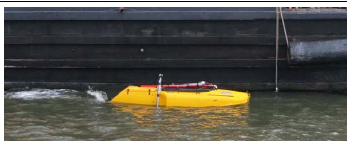
Figure 3.3. The autonomous surface vessel jetyak surveying in front of the barge at the Brooklyn Bridge Park slip.
