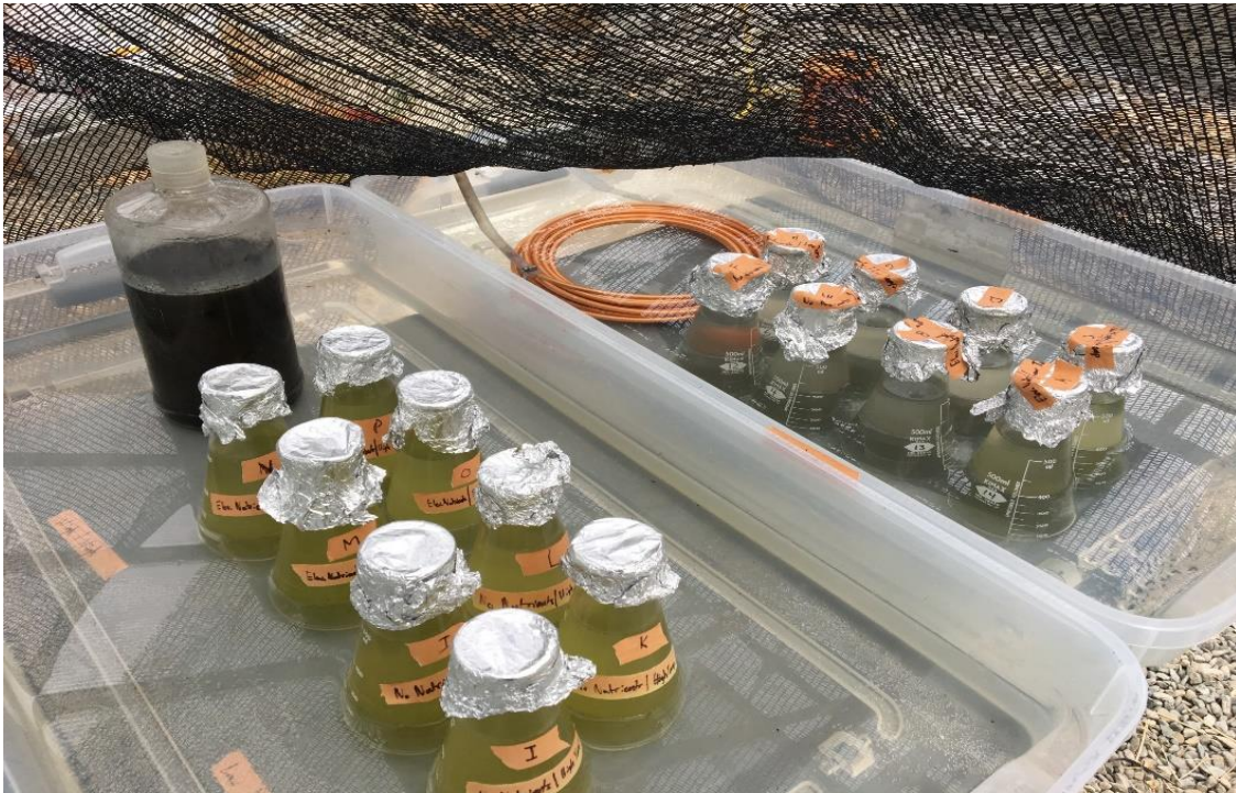
Figure 1: Picture of the experimental setup testing the effects of temperature and nutrients on cyanobacteria concentration. The higher temperature treatment is depicted on the left and the lower temperature is depicted on the right.
