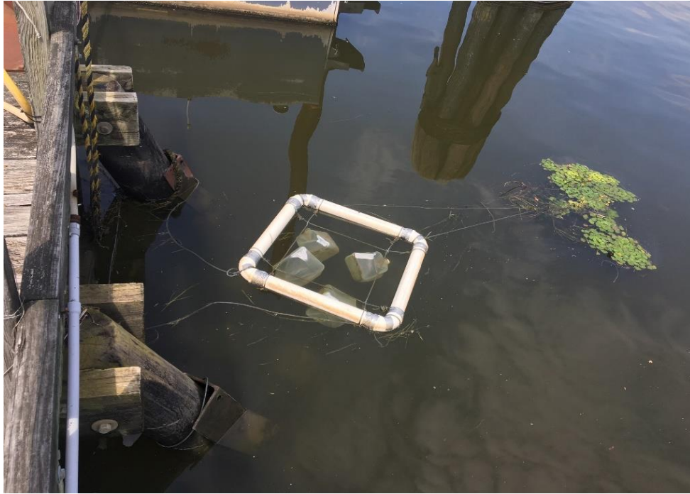
Figure 2: A picture of the experimental rig testing the effects of nutrients and depth on cyanobacteria concentration, placed in the Hudson River at Norrie Point, Staatsburg, NY.
