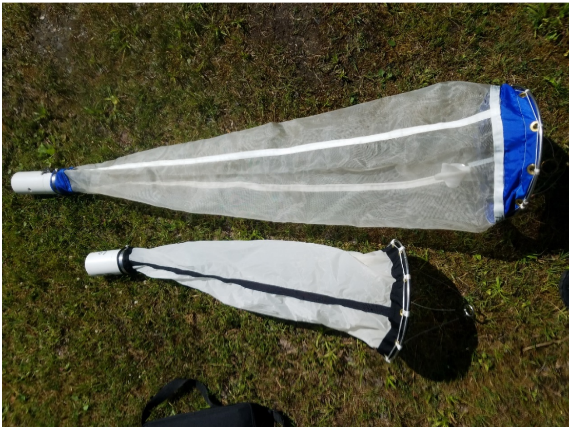
Figure 3: 20 \mu\text{m} (bottom) and 750 \mu\text{m} (top) mesh size nets that were towed horizontally to collect planktonic samples during Summer 2019.
