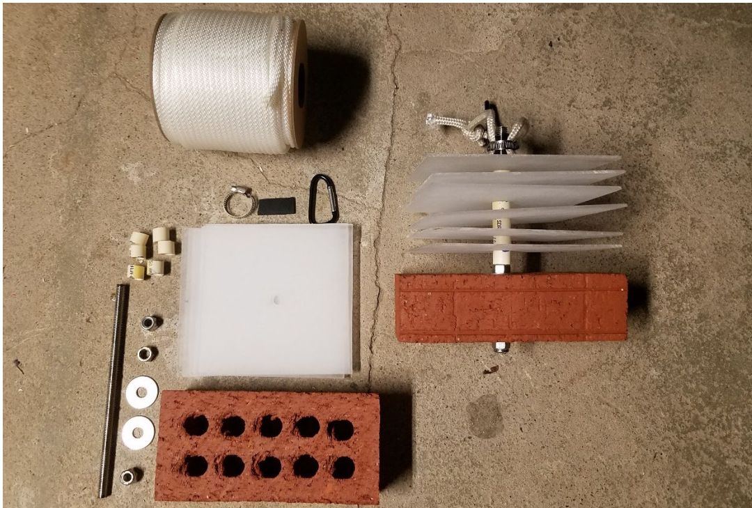
Figure 2: Hester-Dendy settlement plate design used in Summer 2019 sampling.
