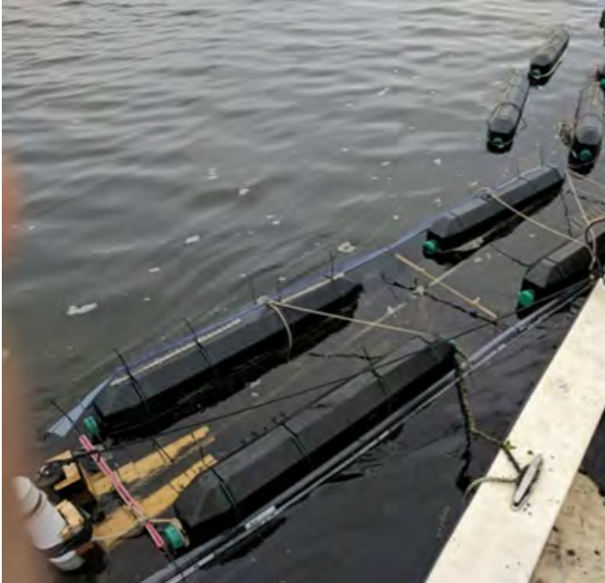
Figure 4.15. Temporary field flume to measure long-term (~40 hours) water filtration by oysters in eight bags on the long line. Note Sontek ADV current meter and Manta datasonde mounted vertically on left end of flume.
