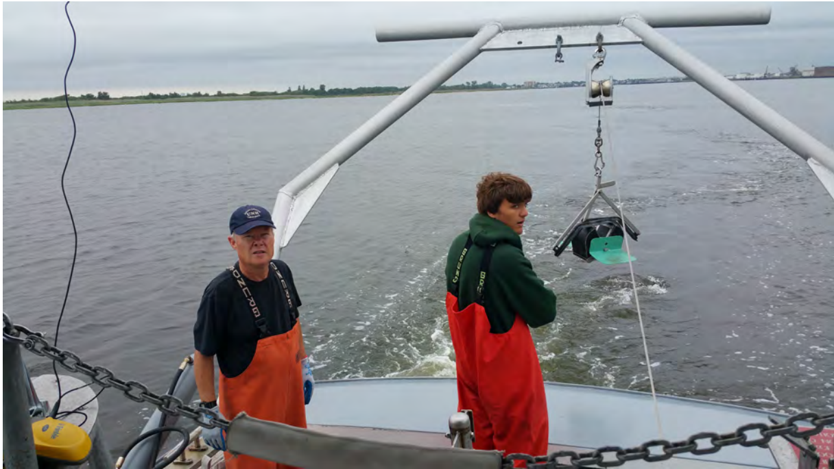
Figure 4.1 Deployment of Van Veen grab used to take pre-construction sediment and benthos samples at project site.
