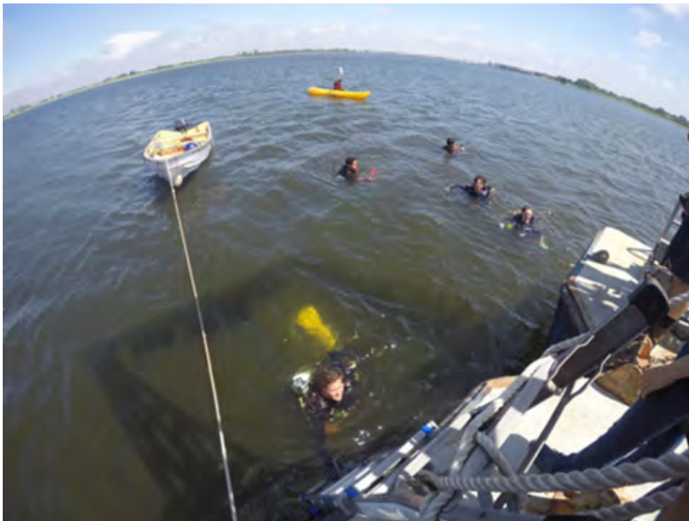
Figure 4.12 Divers retrieving trays containing materials used to construct reef bases and used to characterize biotic communities that developed on the constructed oyster reefs.
