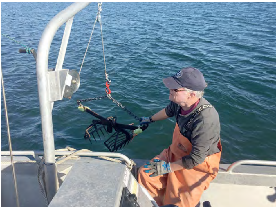
Figure 4.10. Patent tongs used in 2017 to take quantitative samples of the constructed reef bases.
