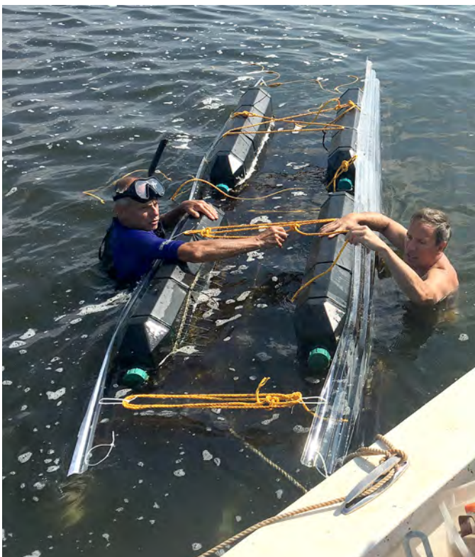
Figure 4.16. Left: Constructing temporary field flume (August 15, 2018) used to measure water filtration by oysters in bags. Right: Field flume anchored in position near channel; note one of two Manta datasondes mounted vertically on each end of flume is visible.
