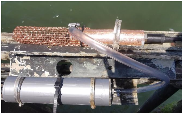
Figure 2 (left): Copper mesh “cage” installed around pump inlet. Credit: Nicole Petersen, Barnegat Bay Partnership
