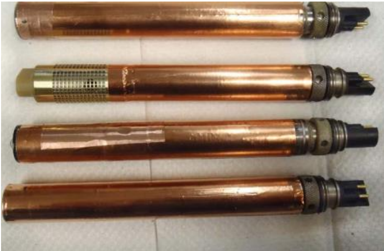
Figure 4: Taping of individual probes (seen here in Copper). Credit: Siddhartha Hayes and Helen Polanco, Hudson River Park River Project.
