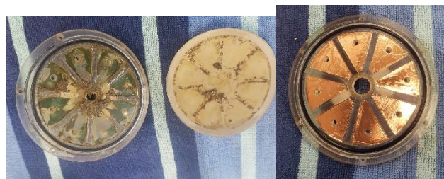
Figure 3 (right): Replacing EnduraFlux membrane and copper tape to pump head. Credit: Nicole Petersen, Barnegat Bay Partnership
