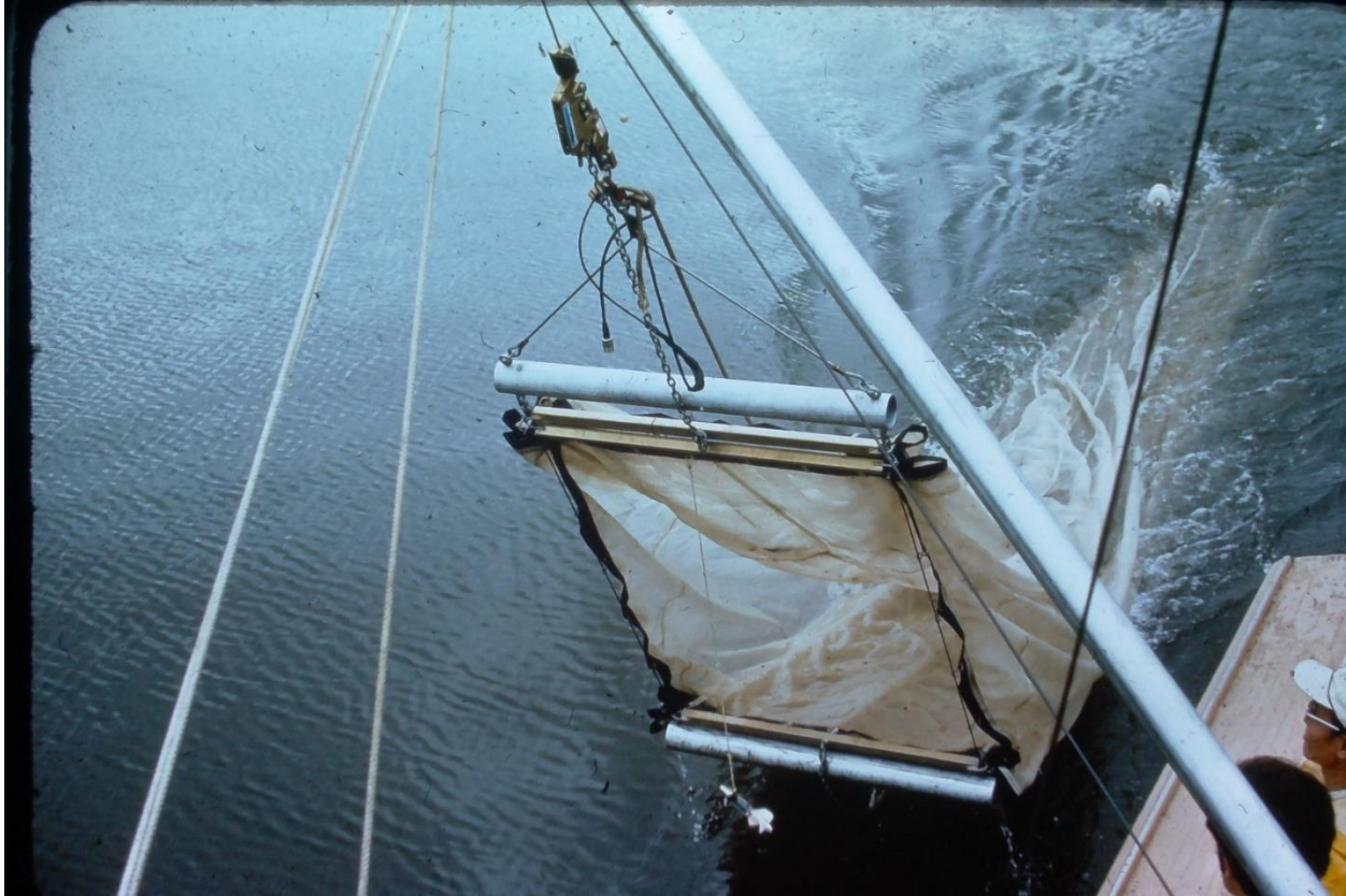
Figure 2-6 1-m 2 Tucker trawl employed to sample shoal and channel strata during LRS program.
