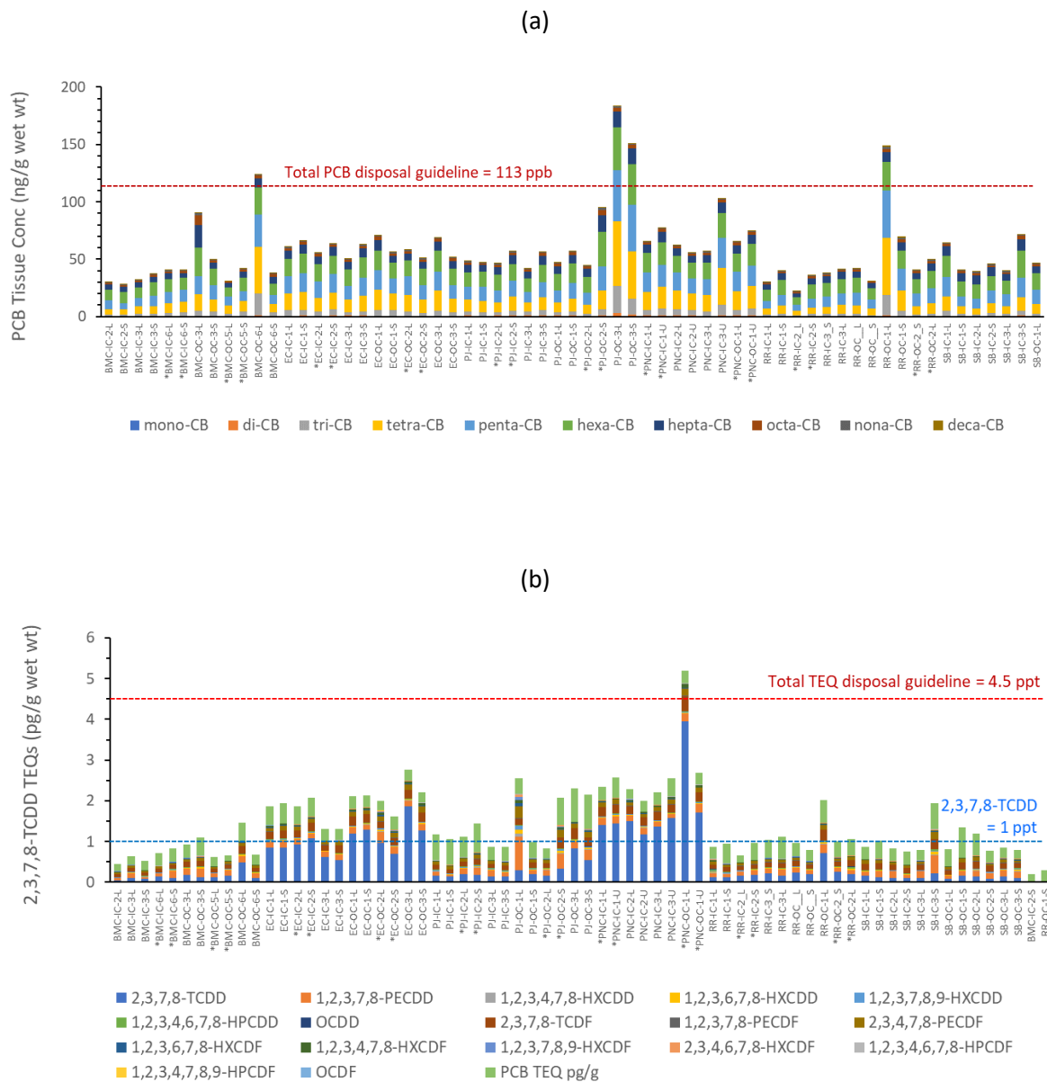
Figure 1. CARP II estimates of tissue concentrations in N. virens for (a) PCB homologs and (b) 2,3,7,8-TCDD Toxic Equivalents (TEQs). Results are presented for 68 sediment samples that were collected throughout NY-NJ Harbor. PCB results were obtained by multiplying 28-day bioaccumulation test results by a factor of 2 (Figure 1a). TEQ results were determined directly from the 28-day bioaccumulation results without adjustment to steady state (Figure 1b). Current dredged material management guidelines for HARS disposal are also presented on the figure for comparison to the bioaccumulation results. (Note: PCDD/F measurements were not given for two of the 68 samples: BMC-IC-2-S and RR-OC-1-S.)
